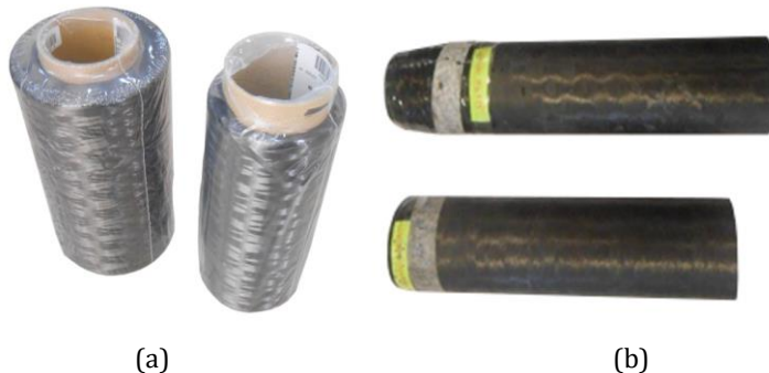
Fig. 4 UMS 40-IMS 65 carbon fiber rolls (a) and composite tubes with fiber orientation of [90/\pm 45/\pm 15/90]_n (b)
