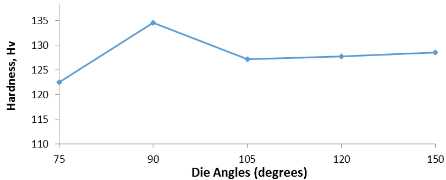
Fig. 4 Plot of Micro-Hardness against Extrudates of various Die Angles
