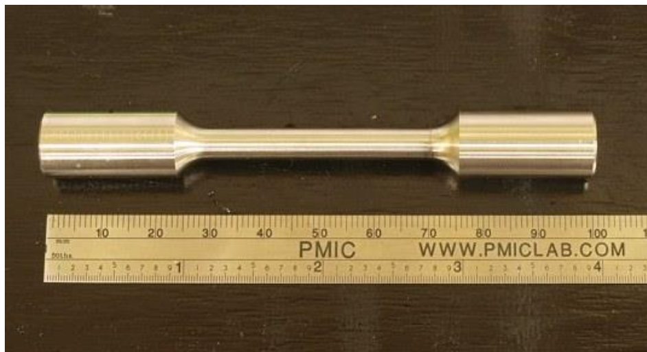
Fig. 2 316L Stainless Steel Tensile Test Specimen
