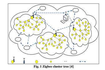
Power management system. This system does not require multiple modes, and allows for reduced functionality devices (or RFDs) that don't require a great deal of ROM or RAM. This comes in contrast to the Bluetooth system, which features multiple modes of operation. Using Zigbee, data is transferred in packets over a distance of up to 230 feet or longer if data is relayed across nodes in a network.
