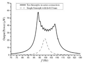
Fig. 13 Generated power level using multiple bimorphs [22]
