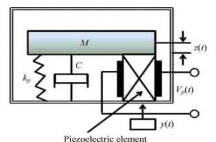
Fig. 11 Simplified equivalent model for the single piezoelectric unit in the array structure
