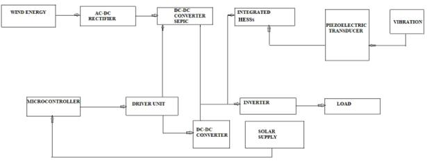
Fig. 15 Block diagram of the Proposed Model of the Integrated System for Energy Harvesting
