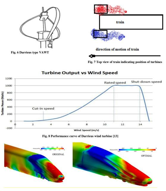
Fig. 9 Pressure distribution near head-coach for optimal and original design [14]
