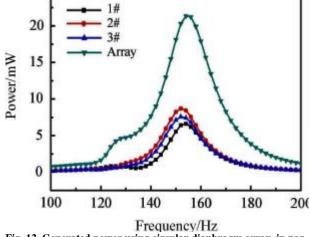
Fig. 12 Generated power using circular diaphragm array in parallel connection [24]
