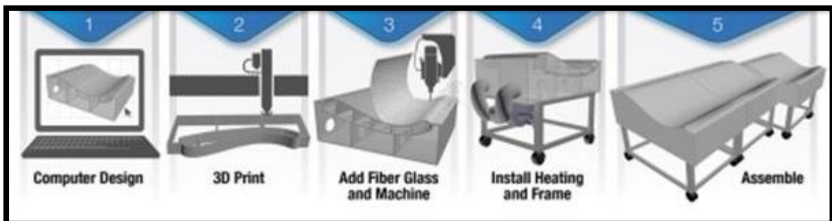
Fig. 7 Process for 3D printing wind turbine blade molds
