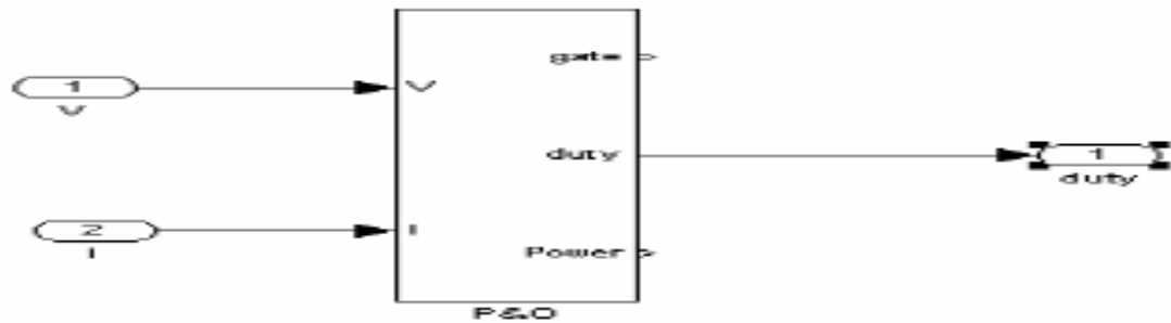
Fig. 13 Perturb and Observe Algorithm Simulink Model for Subsystem
