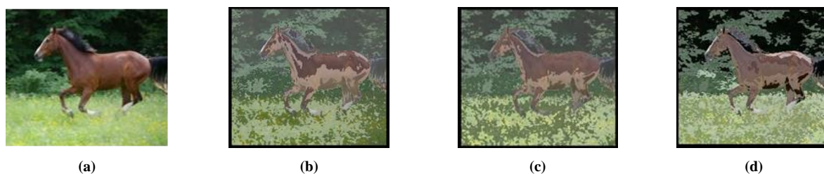
Fig. 6(a) RGB input image (b) segmented image in RGB color space using 5 cluster(c) segmented image in RGB color space using 6 clusters (d) segmented image in RGB color space using 7 clusters
