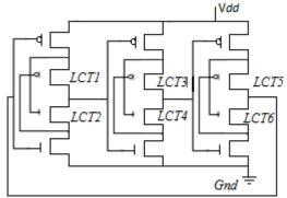
Fig. 5 LACTOR Based Ring Oscillator
