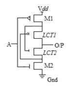
Fig. 4 LECTOR based CMOS Inverter
