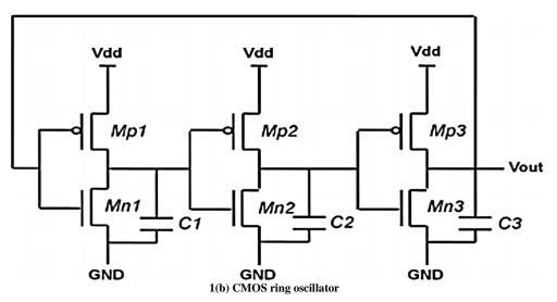
Fig. 1 (a) Symbol diagram of ring oscillator (b) CMOS ring oscillator
