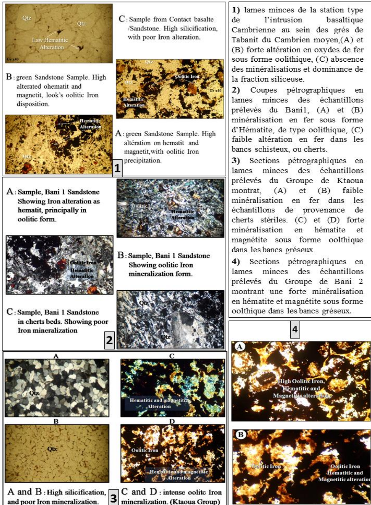
Fig.5 Thin section of O Upper Ordovician mineralized taken samples from Tafilalt Basin of Eastern Anti Atlas of Morocco. (1) Contact zone Tabanit green sandstones – tholeiitic basaltic intrusion of Middle Cambrian showing moderate oolithes iron alteration (A, B) and poor ferruginous mineralization in (C) whit abundance of silica fraction. (2) Bani 1 petrographic observations showing an oolitic hematitic alteration in sandy bands (A, B) and poor iron mineralization in argillic bands (C). (3) Ktaoua group thin sections illustrating a poor iron alteration in argillic or chert bands (A, B) and high ferruginous alteration as hematite and magnetite (oolithic form) in sandy bands. (4) High hematite and magnetite alteration in Bani2 sandstone bands
