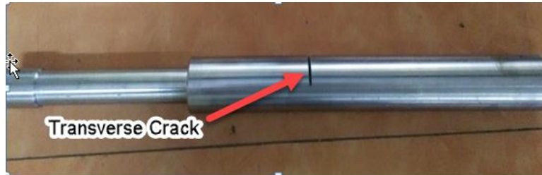
Fig.3 Crack in Shaft
