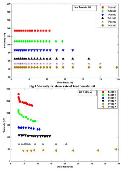
Fig.2 Viscosity vs. shear rate of Ag/ heat transfer oil nanofluid with 0.12% wt (0.011 %Vol.)
