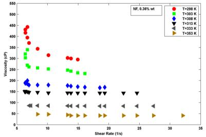
Fig.3 Viscosity vs. shear rate of Ag/ heat transfer oil nanofluid with 0.36% wt (0.044 %Vol.)
