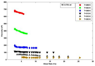
Fig.4 Viscosity vs. shear rate of Ag/ heat transfer oil nanofluid with 0.72% wt (0.171 %Vol.)
