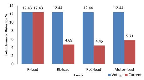
Fig.18. Graph shows the THD for 31-level at variable loads
