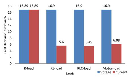
Fig.16. Graph shows the THD for 7-level at variable loads
