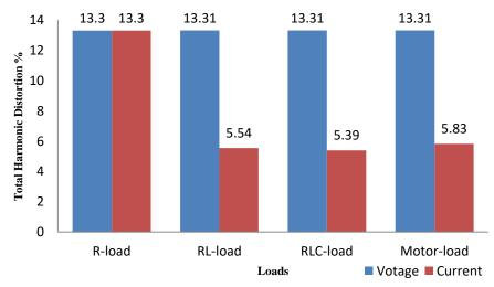
Fig.17. Graph shows the THD for 15-level at variable loads
