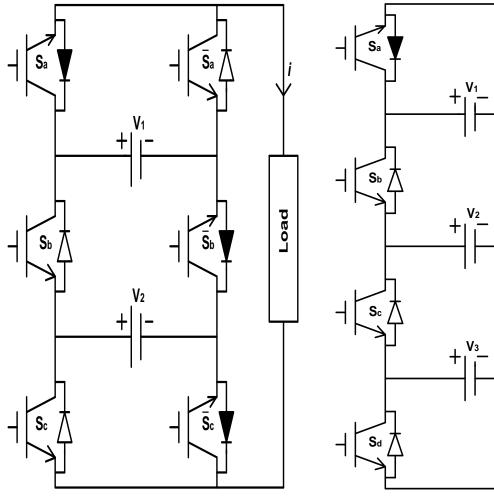
Fig.1.Seven level converter
