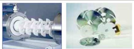
Fig. 6 Agitator shaft of Dynomill (left) and agitator discs in the Dynomill (right)
