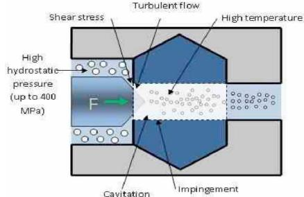
Fig. 7 Various physical phenomena simultaneously affecting a fluid during high pressure homogenization
