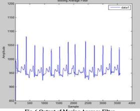
Fig. 6 Output of Moving Average Filter
