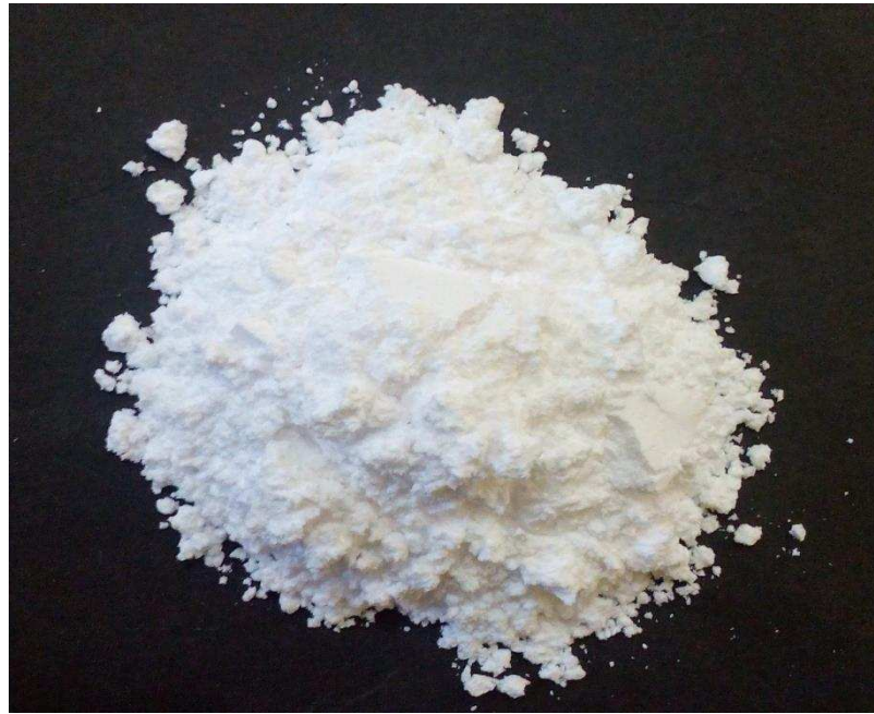
Fig. 2 HAp powder obtained by Calcium Hydroxide and Ortho Phosphoric Acid by precipitation Route
