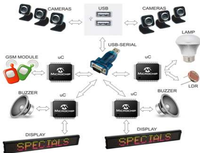
Fig.1 Hardware Framework for SCADA System
