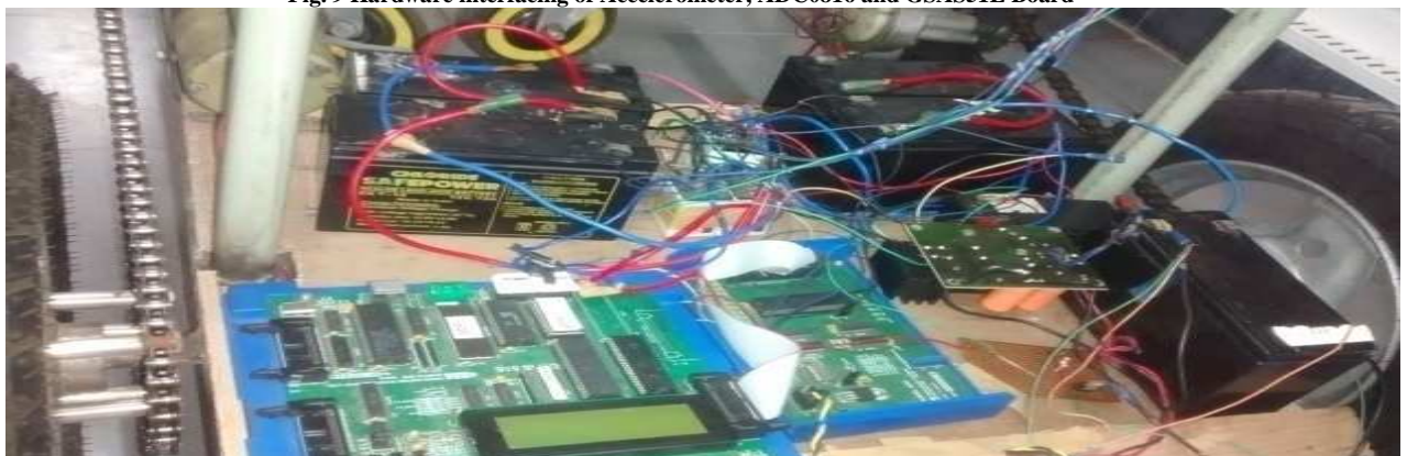
Fig. 10 Complete hardware interfacing of Accelerometer controlled wheelchair
