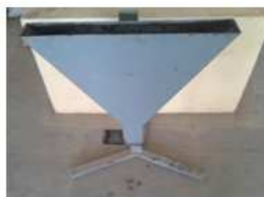
Fig. 1(b) V-Funnel Test
