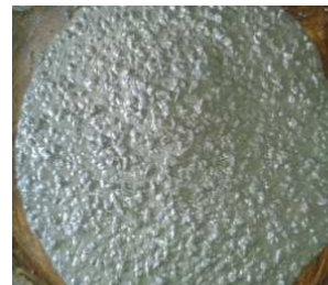
Fig. 1(a) Slump flow & T50 sec Test
