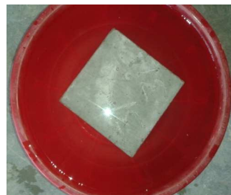
Fig. 5 Chloride Penetration Test
