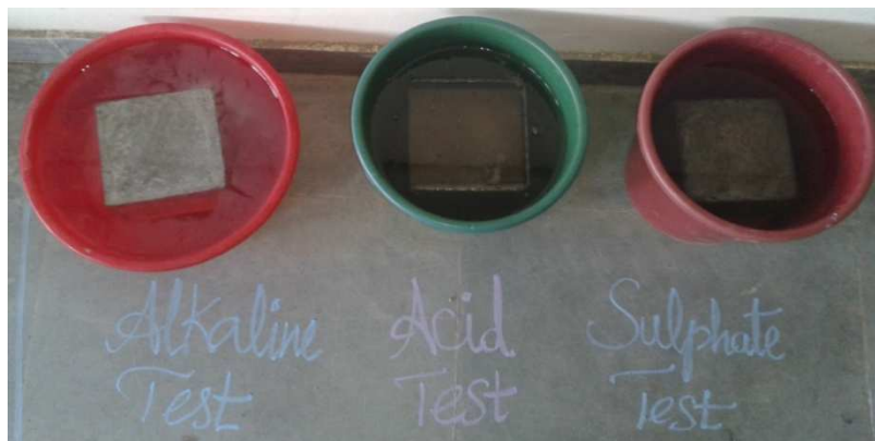
Fig. 2 Alkaline, Acid and Sulphate Test
