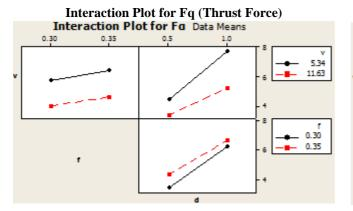
Fig. 8 Interaction Plot for Thrust Force Among Speed, Feed and Depth of Cut
