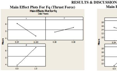
Fig. 6Thrust Force V/S Speed, Feed and Depth of Cut
