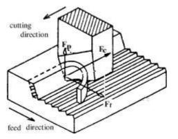
Fig. 3 Mechanism of Shaping Operation [15]
