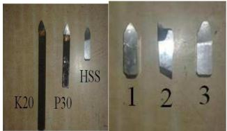
Fig. 5 Different Tool Materials& Shapes
