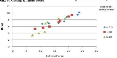
Fig. 12Effect of Tool Material on Cutting & Thrust Force
