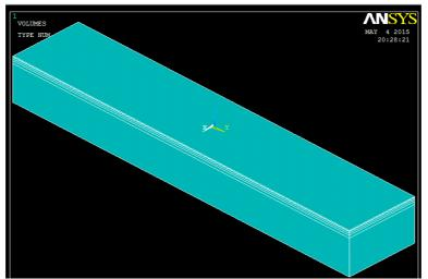
Fig. 2 3D model of six layered flexible of pavement modelled as volume with Solid element as 20-node-186
