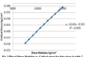
Shear Modulus vs Critical Stress
