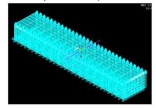
Fig. 9 3D model of with ends restrained and point load ready to analyzed
