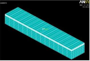
Fig. 7 3D model of various layers of pavement meshed by volume sweep for finite element analysis
