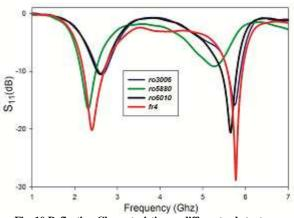
Fig. 10 Reflection Characteristics on different substrates
