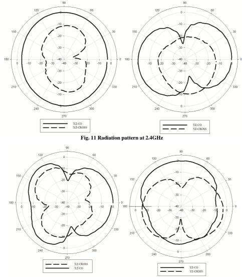
Fig. 12 Radiation Pattern at 5.8GHz
