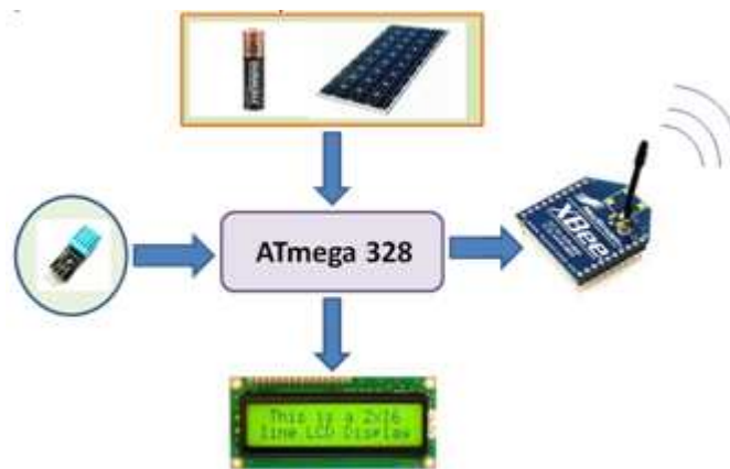
Fig. 2 Wireless sensor network node block diagram (Sensor Node Architecture)
