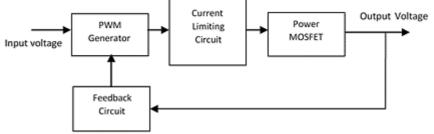
Fig. 12 Block diagram of the Electronic Circuit
