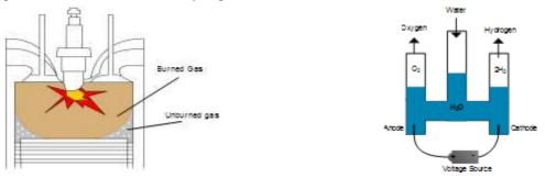
Fig.1 Flame Propagation in the chamber
