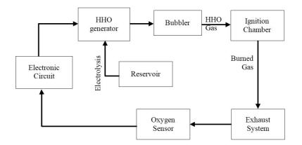
Fig. 13 Block diagram of the Complete System
