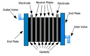
Fig. 5 Cross Sectional view of the proposed HHO generator
