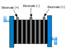
Fig. 7 HHO generator with three electrodes applied
