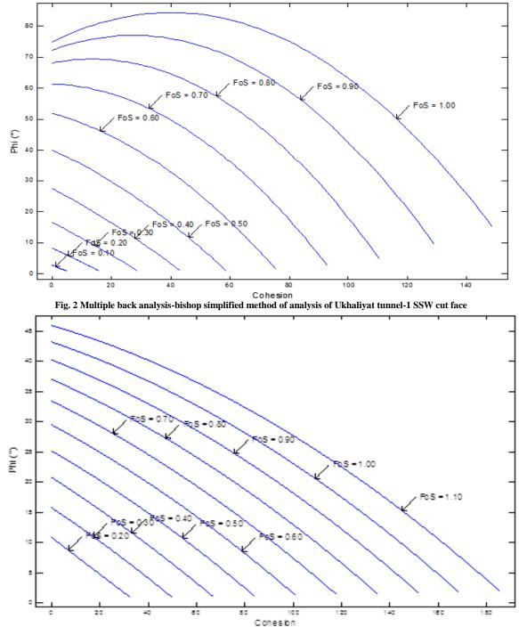
Fig.3 Multiple back analysis-bishop simplified method of analysis of Khokhariyanal tunnel-2 SSE cut face
