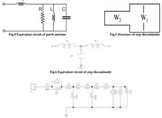
Fig.7 Equivalent circuit of proposed antenna
