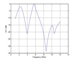
Fig. 8 Simulated return loss of the proposed antenna
