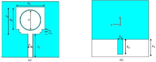
Fig.1 Antenna configuration (a) front (b) back view
