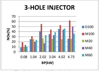
**Fig -13**: Variation of  $NO_X$  with brake power
