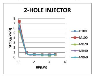
FIG -6: VARIATION OF SPECIFIC FUEL CONSUMPTION WITH 2 NO OF HOLES
