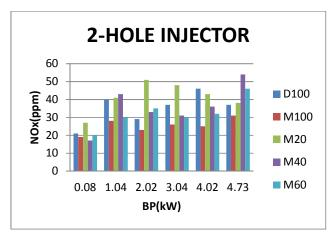
**Fig -12**: Variation of  $NO_X$  with brake power
