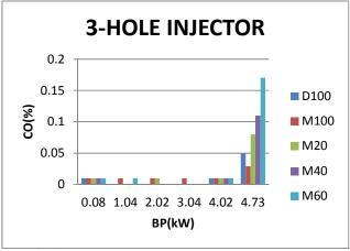
Fig -9: Variation of carbon monoxide with brake power.
