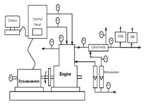
FIG -3: LINE DIAGRAM OF EXPERIMENTAL SET UP
