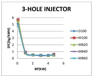
**fig-7**: Variation of specific fuel consumption with 3 no of Holes
