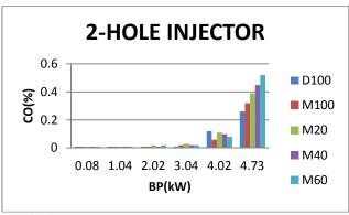
Fig -8: Variation of carbon monoxide with brake power.
