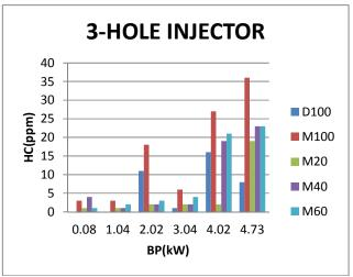
Fig -11: Variation of hydrocarbon with brake power.
