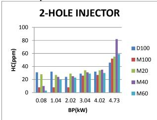
Fig -10: Variation of hydrocarbon with brake power.
