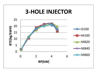
FIG -5: VARIATION OF BRAKE THERMAL EFFICIENCY WITH 3 NO OF HOLES
