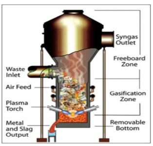
Fig. 5: Westinghouse Plasma Corporation's proprietary plasma gasification vitrification reactor
