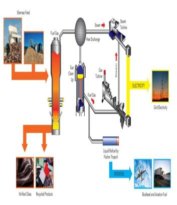
Fig 1-plasma gasification process.
