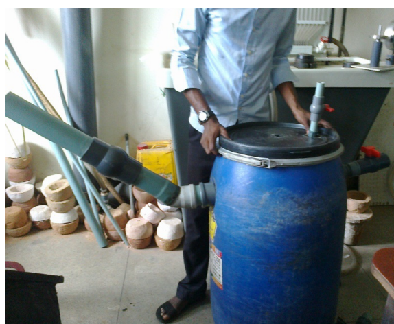
Plate 2: The Slurry Inlet and the Outlet
