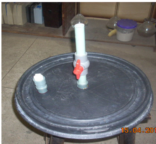
Plate 3: The Gas Outlet with the fixed Cover
