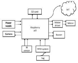
Fig2: Block diagram of proposed system
