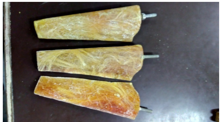
Fig Glass fiber with epoxy blades with bolt in bottom
