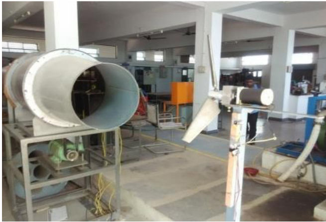
Fig wind tunnel with wind turbine made of aluminum blades
