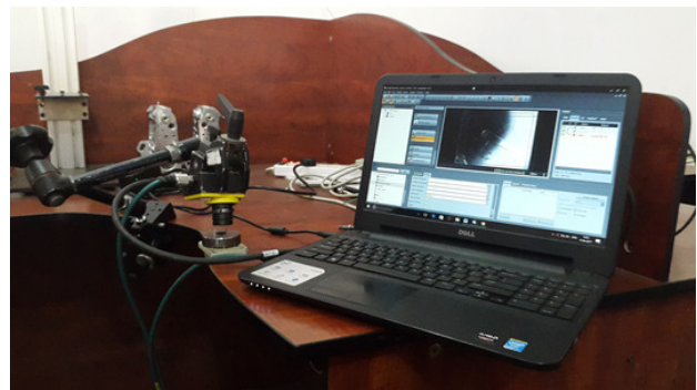
Fig 4: Experimental setup for Vane plate placement error detection
