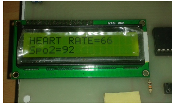
Fig. 10 Heart Rate and Spo2 % of Patient Indicated on LCD
