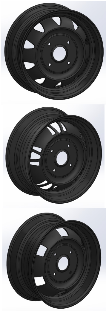
Fig. 4: Optimized pattern of the wheel rim having different topology
