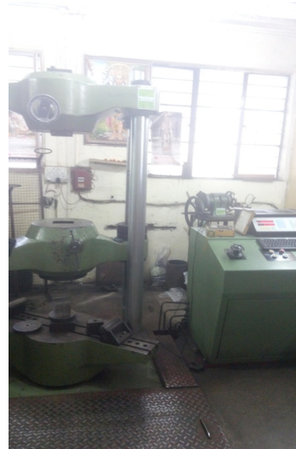
Fig.10 Universal Testing Machine Experimental set up For Excavator Pins
