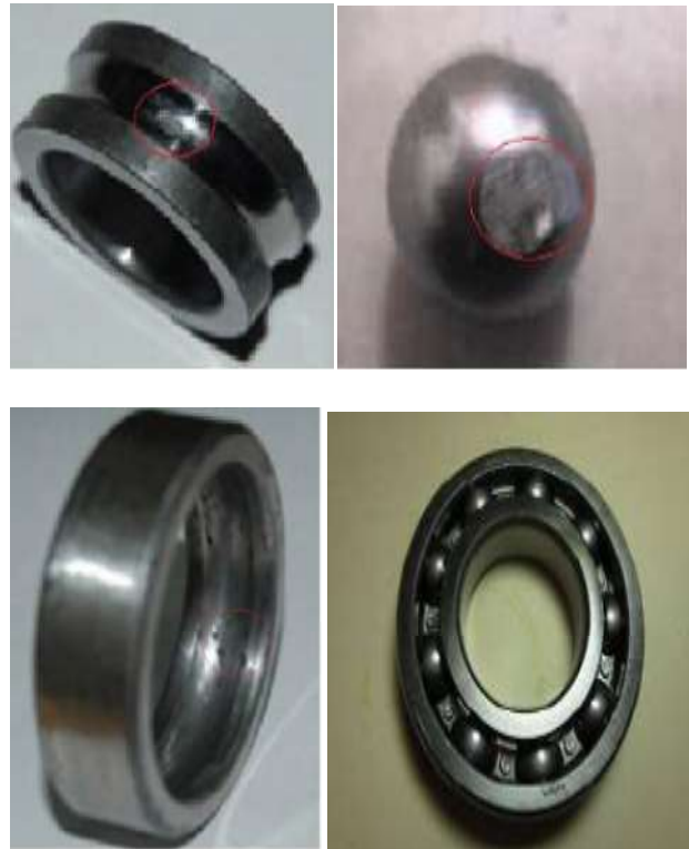
Fig.4. (a) Spall at inner race (b) Spall at ball (c) Spall at outer race (d) Healthy bearing
