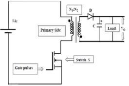
Fig.2. Basic Topology of Fly-Back Converter.
