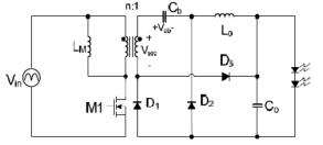
Fig.11. Proposed single stage PFC forward flyback converter circuit
