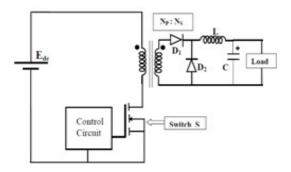
Fig.3. Basic forward converter topology
