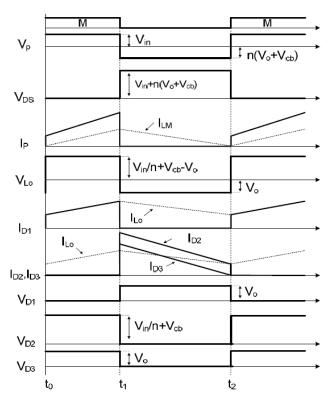
Fig.13. Key waveforms of the proposed forward – flyback converter
