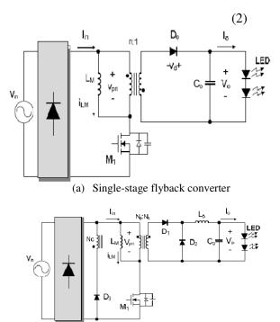
(a) Single stage forward converter Fig 8 Conventional single stage PFC converter circuits
