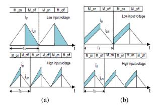
Fig.12. Primary and magnetizing currents of forward-flyback converter according to the input voltage. (a) Without balancing capacitor (b) with balancing capacitor
