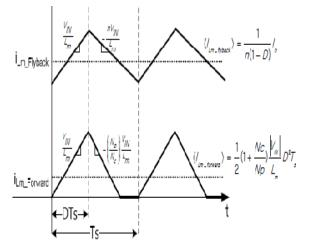
Fig.9. Transformer magnetizing inductor currents of conventional flyback and forward converters
