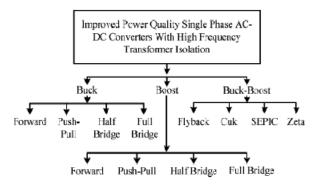
Fig.1 Classification of AC-DC Converter
