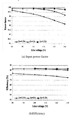
Fig.7. Experimental efficiency and input power factor.
