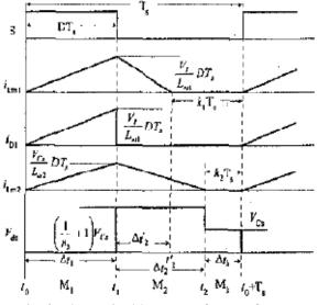
Fig.6. Theoretical key waveforms of proposed converter.
