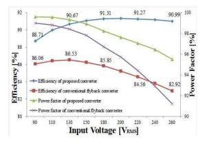
Fig.14. Comparisons of efficiency and power factor between flyback and proposed forward-flyback converter
