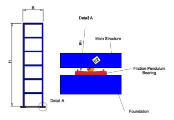
Figure 3. Friction pendulum bearing under the analyzed frame.  $104 \end{tabular}$
