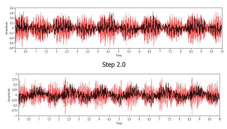
Figure 5. Acceleration  $[m/s^2]$  of top of the frame (red line) and the table (black line) in time domain [s]
