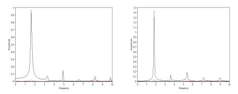
**Figure 6.** FFT of acceleration of top of the frame for steps from 0.5 to 5.5, black line - table, red line - frame.
