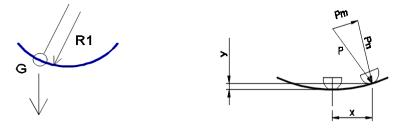
Figure 2. Concept of pendulum on the left, forces acting on the friction pendulum bearing on the right
