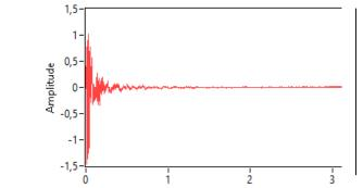
In the figure 4 response of the model structures under free vibration is presented. Natural frequency is 6.86 Hz.
