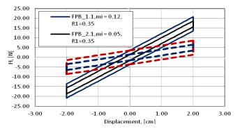
Figure 8. Response curves of the friction pendulum bearing for fixed dynamic friction coefficient 'mi' and sliding surface curvature radius 'R1'
