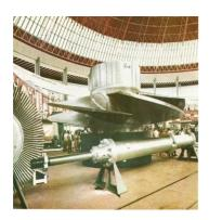
Figure 16 The Kaplan rotor
