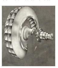
Figure 11 The rotor of a exhauster
