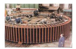
Figure 21 The bulb generator rotor
