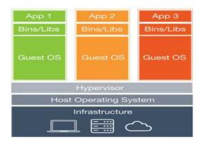
**Figure 1: Virtualization Architecture**
