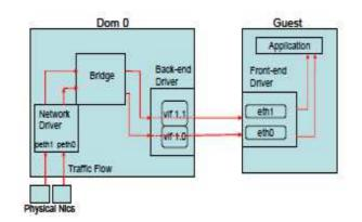
Figure 6: XennetworkI/O Processing[29]
