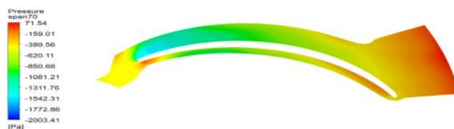
Figure 11: Static Pressure Contour 70% at 10000 rpm
