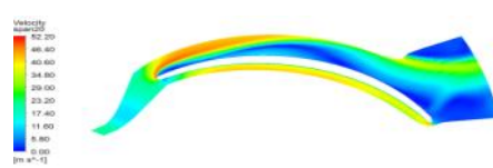
Figure 6: Velocity Contour 20% at 10000 rpm
