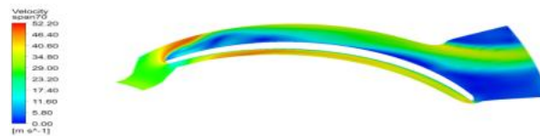
Figure 8: Velocity Contour 70% at 10000 rpm
