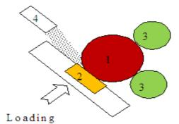
Figure 2: Ball-Cratering Tribometer Schematic Diagram 1. Tungsten Ball 2. Specimen 3. Shaft 4. Slurry
