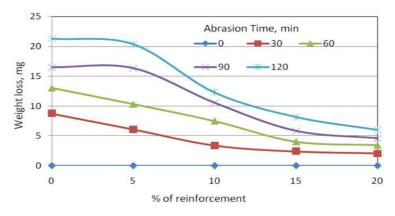
Figure 6: Variation of Mass Loss with % of Reinforcement for Al/TiB<sub>2</sub> Composites Abraded by Alumina Slurry for Different Sliding Duration
