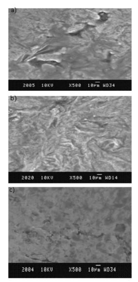
Figure 7: Worn-Out Surface Ball-Crater Morphology of (a) Al 6061 Alloy, (b) Al/5 % Tic and (c) 20% Tic Samples Abraded by the Aluminum Slurry
