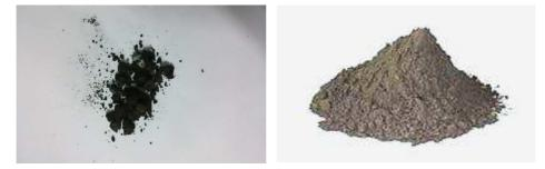
Figure 1: CuO Nanoparticles (a) Before Sintering (b) After Sintering
