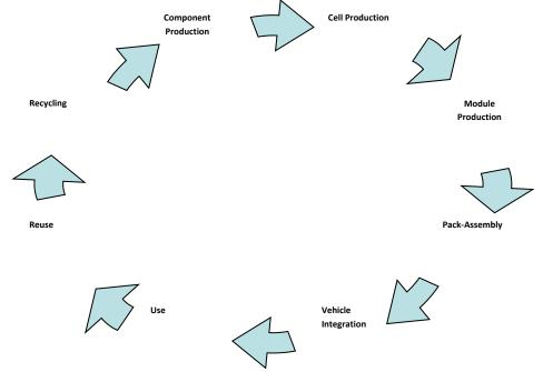
Fig. 1: Stages in Electric Car Battery Value Chain
