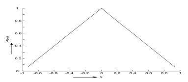
Figure 3: Triangular Amplitude Distribution along the Line Source
