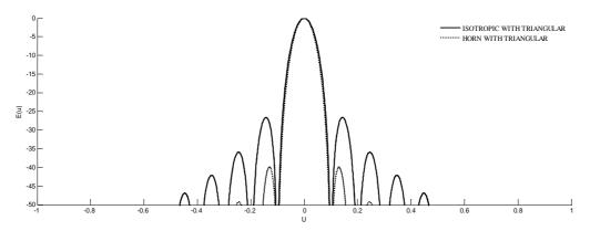
Figure 12: Synthesized Isotropic Arrays with and Without Waveguide for N=40
