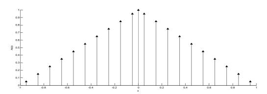
Figure 5: Triangular Amplitude Distribution with Discrete Locations of N=20
