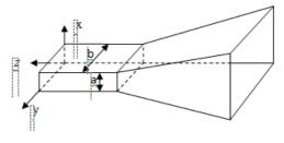
Figure 1: Pyramidal Horn Antenna
