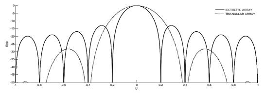
Figure 7: Triangular Amplitude Distribution with Isotropic Array for N=10
