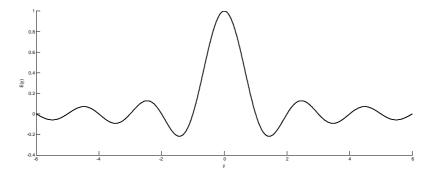
Figure 2: Rectangular Plot of Horn Antenna (Element Pattern)
