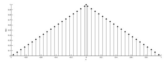
Figure 6: Triangular Amplitude Distribution with Discrete Locations of N=40
