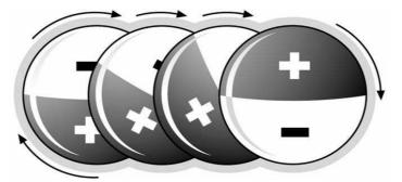
Figure 2.4: Rotation of Gyricon Beads during Charge Transition
