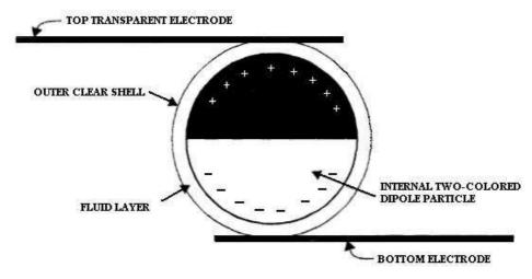
Figure 2.1: Schematic of an Electronic Ink Particle
