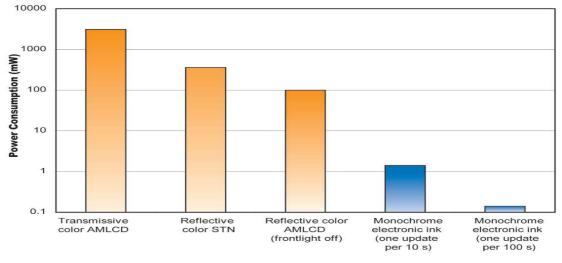
Figure 4.2: Comparison of Display Power Consumption LCD and Electronic Ink Display Technologies for Two Display Formats
