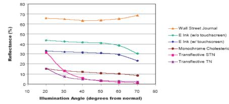
Note: Reflectivity measurements were taken with the detector at the display normal (0°) using a collimated source positioned at angles ranging from 20° to 70°.
