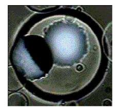
Figure 2.2: Photomicrograph of Electronic Ink
