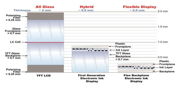
Figure 4.3: Comparison of Display Cell Structure between Conventional LCDs and Electronic Ink Displays
