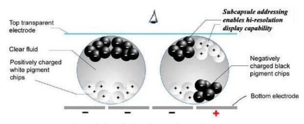
process, the black particles appear at the top of the capsule, which now makes the surface appear dark at that spot.
