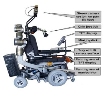
Fig. 2. The Care-Providing robot FRIEND [16]
