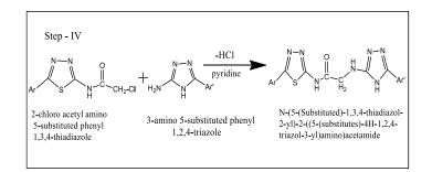
A mixture of 2-Chloroacetyl amino, 5-substituted phenyl, 1,3,4-thiadiazole(0.001mole) and 3-amino 5-substituted phenyl 1,2,4-triazole(0.001mole) using solvent DMF (15ml) in presence of pyridine, was heated manually for time mentioned in table no.4. The mixture was allowed to cool and crushed ice was added. The precipitate was filtered and solid was dried and recrystallized from ethanol. Purity of product was checked by TLC using solvent system (Ethyl acetate: n-hexane 7:3).
