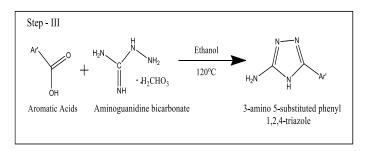
A mixture of Aminoguanidine bicarbonate (0.01 mole) and Aromatic acids (0.01 mole) in ethanol was warmed manually, till the bubbles of carbon dioxide was evolved. The mixture was irradiated under microwave at power and time mentioned in table no.3. The solution was evaporated to collect the solid. The solid was recrystallized with ethanol. Purity of product was checked by TLC using solvent system (Benzene: Methanol 7:3).
