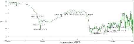
Fig. 2a: FTIR spectra of Lornoxicam
