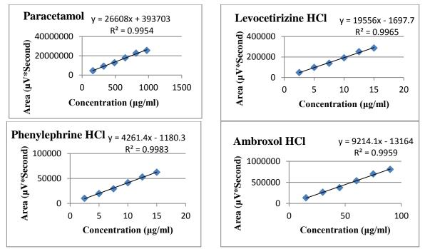
Fig 4: Calibration curve of Paracetamol, Levocetirizine HCl, Phenylephrine HCl and Ambroxol HCl
