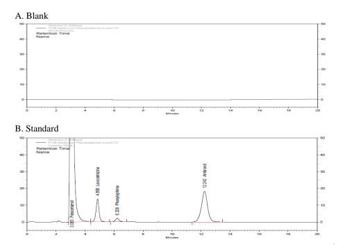
Fig. 5: Chromatogram of blank and Standard for specificity
